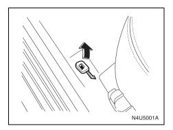
To open the fuel filler door, pull up on the fuel filler door release lever located on the floor to the left of the driver's seat.
